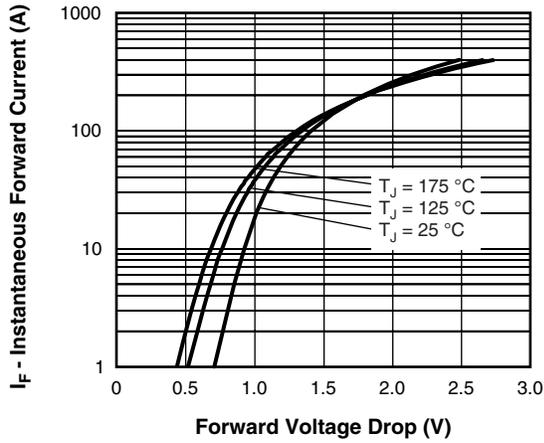
Fig. 1 - Maximum Forward Voltage Drop Characteristics (Per Diode)
